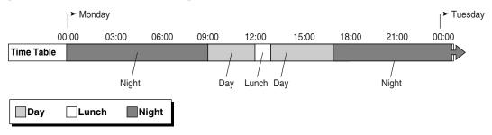
Note that time service modes can be arranged as they are needed (for example, night mode can occur in the morning and afternoon, if necessary) and not all time service modes need to be used in a time schedule. Also note that day mode or night mode resumes automatically when lunch mode ends.
