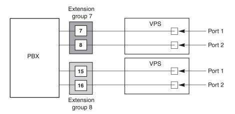
This pattern uses 2 Panasonic KX-TVA50/KX-TVS50/KX-TVS90 VPSs, which can be connected with 4-conductor wire to 4 extension jacks of the PBX.
