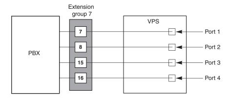
This pattern uses a Panasonic KX-TVA series VPS version 2.0 or later, where up to 4 extensions can be connected to one VPS.
